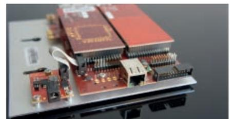
beroNet VoIP Gateways can be assembled with up to 2 modules and are very flexible. They can be easily adapted to different customer requirements.
